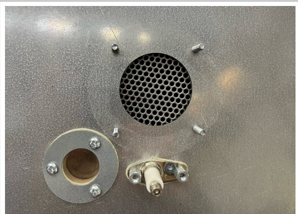
Figure 30 - The grid in front of the burner
