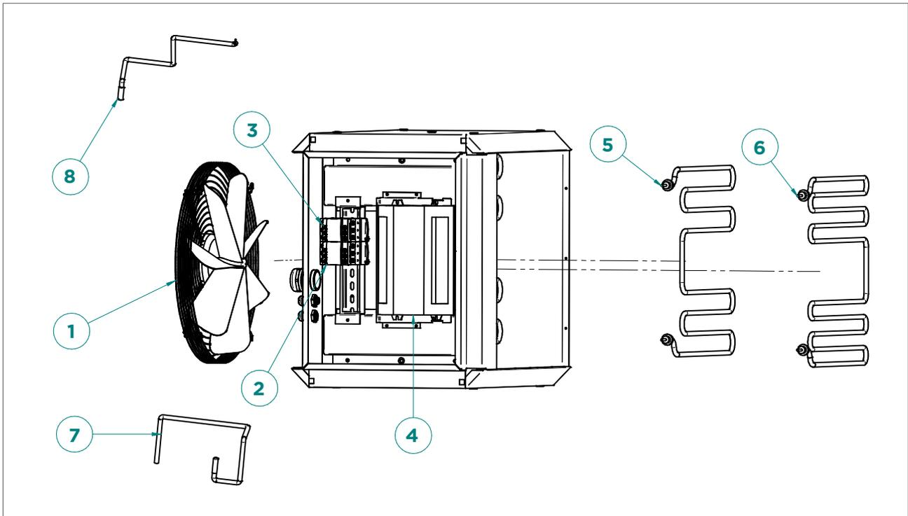
Figure 16 - Exploded view of the EH
