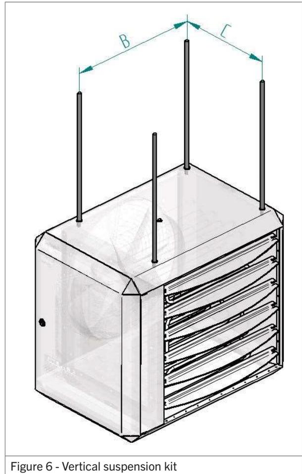
Figure 6 - Vertical suspension kit
