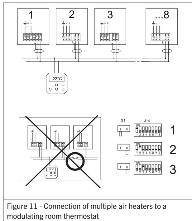
Figure 11 - Connection of multiple air heaters to a modulating room thermostat
