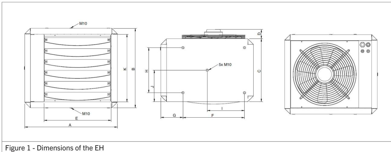
Figure 1 - Dimensions of the EH
